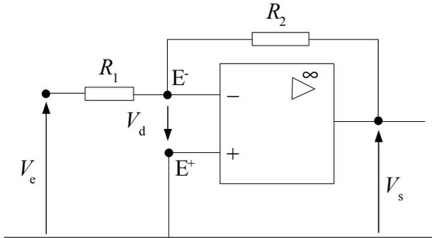
$$V_s = -\frac{R_2}{R_1} V_e \Rightarrow A_v = \frac{V_s}{V_e} = -\frac{R_2}{R_1} \quad A_v : \text{coefficient d'amplification}$$
